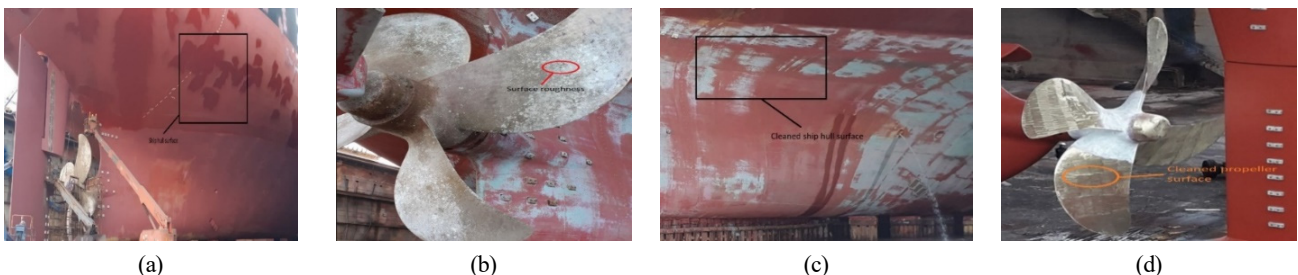
Fig. 10 Actual surface condition of ship hull and marine propeller before/after coming to dock: (a) ship hull (before), (b) propeller (before), (c) ship hull (after), and (d) propeller (after)
