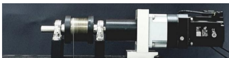
Fig. 4 AC servomotor and wire drum for towing the submerged body
