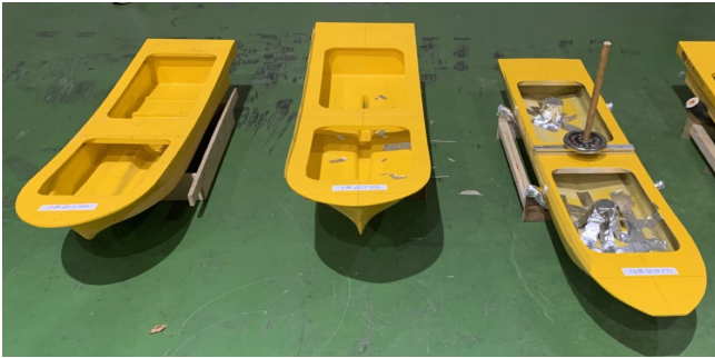
Fig. 2 Picture of experiment models (From the left, 3 G/T class, 7 G/T class, 10 G/T class)
