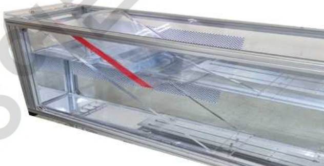
Fig. 2 Inclined OWC installed in the two-dimensional mini wave tank
