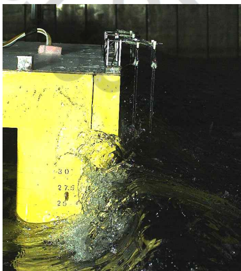
Fig. 12 Extreme upwell and largest upwell for RW02 and R-RW02
