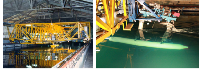
Fig. 9 Towing tank and carriage at KRISO (left) and VPMM tests of underwater vehicle in this study (right)
