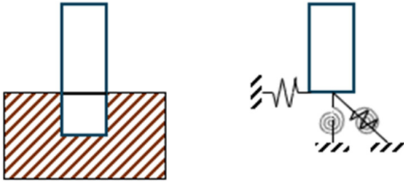
Fig. 7 Coupled spring model to consider the effect of the foundation (Jung et al., 2015)
