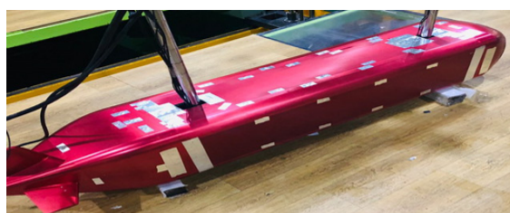
(a) Profile of underwater vehicle (model test)
